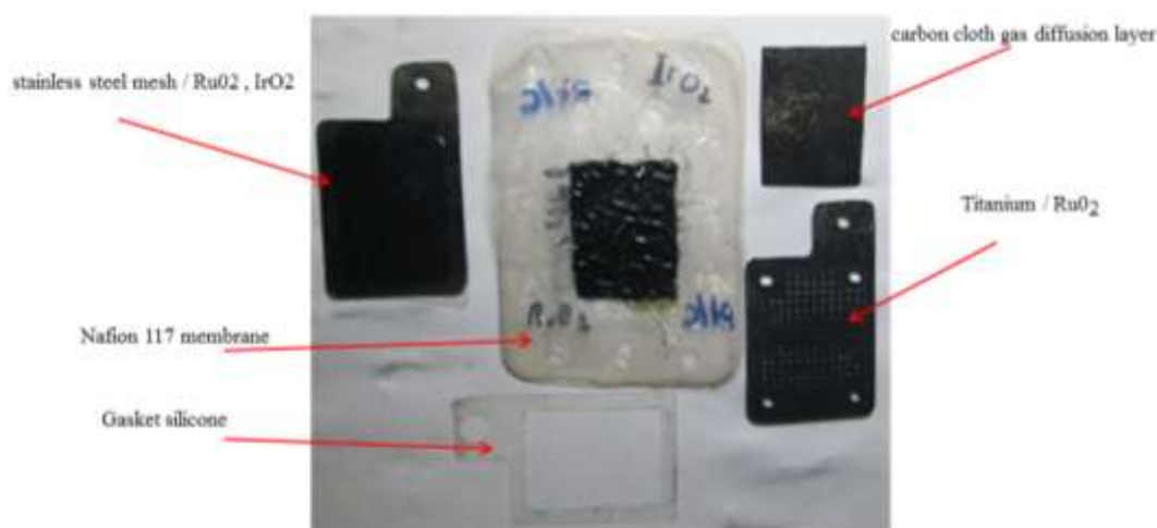
Figure 3. SPE electrolyzer Components
